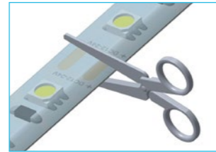
Cut the LED strip in cutting points
