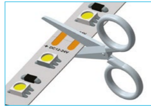
Cut the LED strip in cutting points
