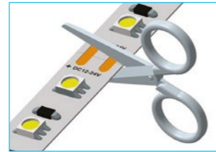
Cut the LED strip in cutting points
