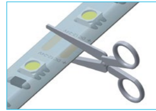
Cut the LED strip in cutting points
