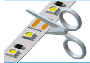
Cut the LED strip in cutting points
