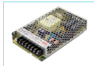
Order code: LRS-150-24 85-132VAC/170-264VAC by switch DC24V 150W IP20, global certification Indoor use only.
